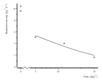
**Figure B1** Concentration-effect curve of the effect of 3,5-dichlorophenol on activated sludge respiration rate.
